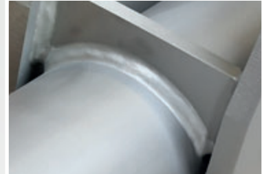
▲ Weld seam according to execution class EXC3
