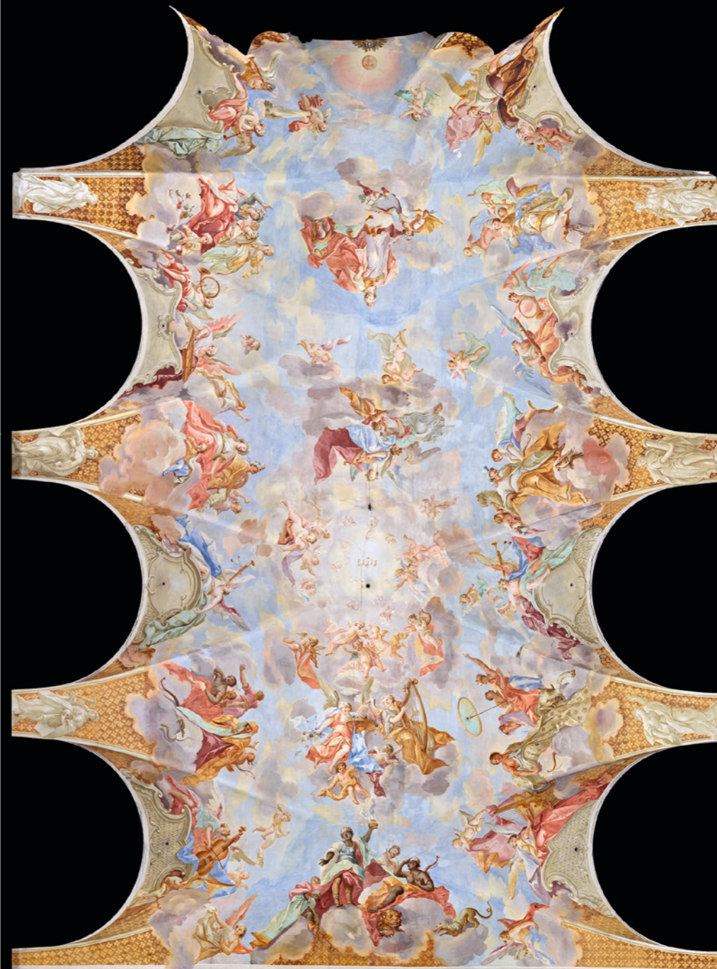
Weißenaue, Abbey Church St. Peter and Paul. Digitally developed surface with ortho-projected choir vaulting. (Original at a scale of 1:10 with 400 dpi resolution)
