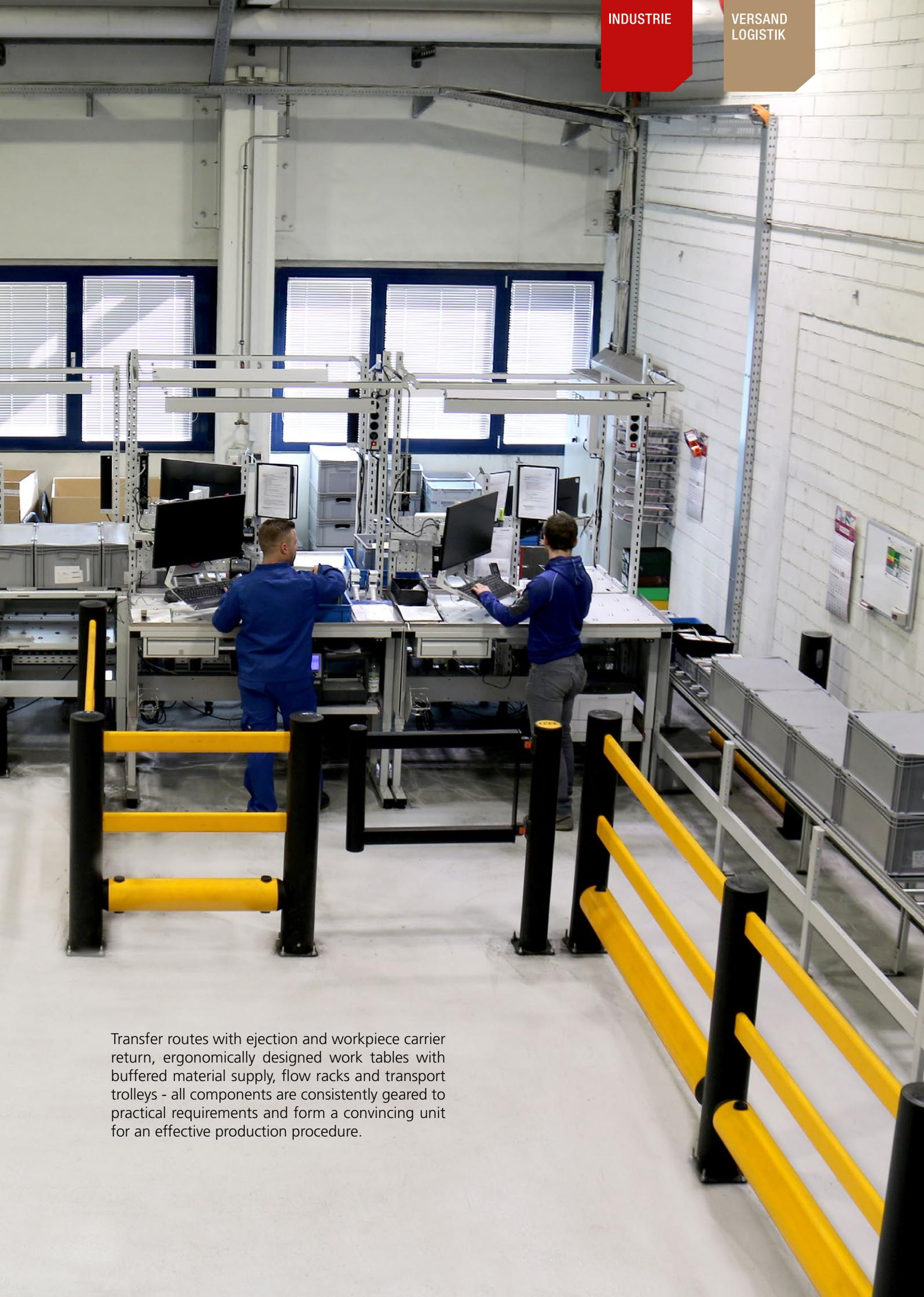
Transfer routes with ejection and workpiece carrier return, ergonomically designed work tables with buffered material supply, flow racks and transport trolleys - all components are consistently geared to practical requirements and form a convincing unit for an effective production procedure.
