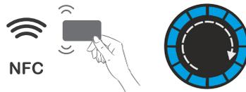
1. Hold the Master RFID card against the RFID reader. When the card is recognised, the illuminated ring rotates once to the right.
