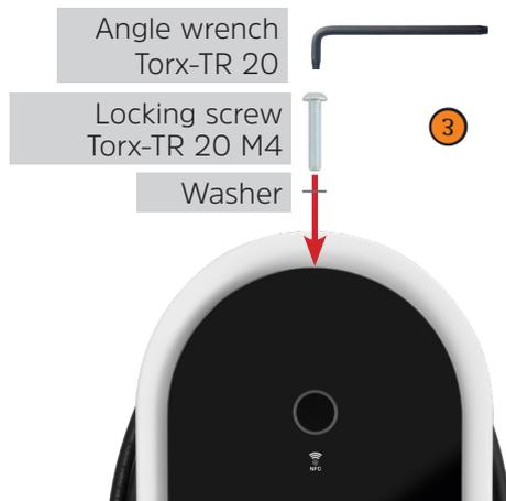
3. Now screw the Torx-TR 20 M4 locking screw and washer (included in the scope of delivery) into the threaded bush above the front glass panel using the Torx-TR 20 angle wrench.
