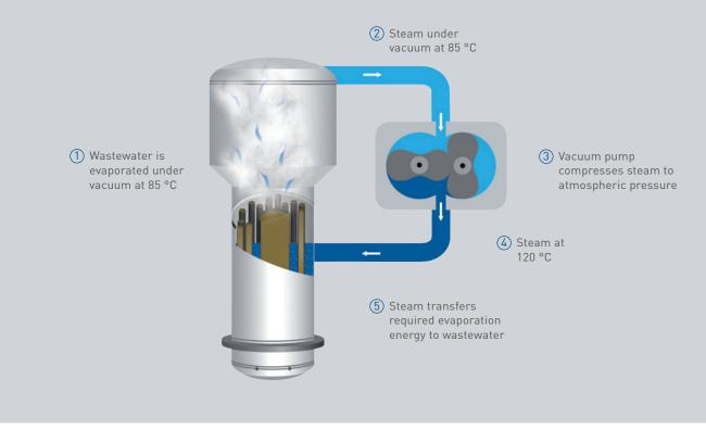
Thanks to energy recycling the VACUDEST<sup>®</sup> process is a forerunner regarding optimization of energy efficiency and reduction of operating cost.
